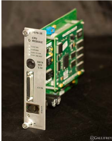
2070-1E Module Front Panel View
