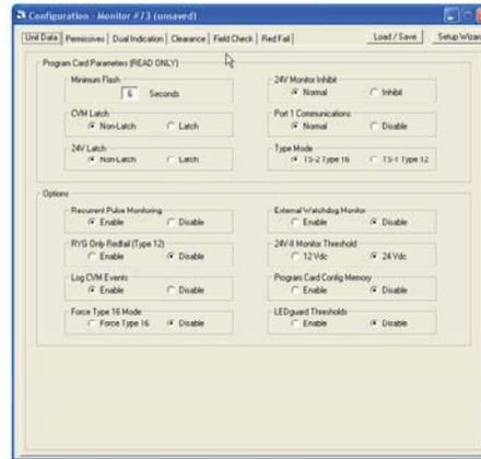
Sometimes it is not good enough to determine the monitor programming visually by checking the Program Card and front panel switches. The Monitor Configuration display will show the complete programming of the monitor including all Program Card parameters as well as switches and internal option jumpers.
