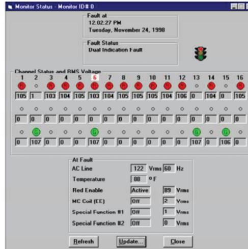
View a display that graphically displays signal On/Off states as well as the RMS voltage at each field terminal and at the AC Line input. It is like having a 48+ channel digital voltmeter connected to the cabinet 24 hours a day, 365 days a year.
