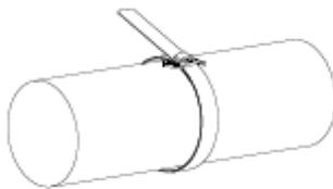
4. Position the band on the object you are clamping. Pull the wrapped band hand-tight. Slightly bend the tail up to keep the clamp in place
