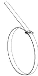
3. If desired, you may preform a clamp in the same fashion as step 2, or use a ULTRA-LOK® preformed clamp in place of a ULTRA-LOK® Free-End
